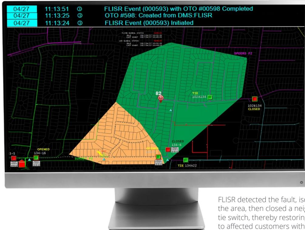
FLISR detected the fault, isolated the area, then closed a neighboring tie switch, thereby restoring power to affected customers within seconds.
