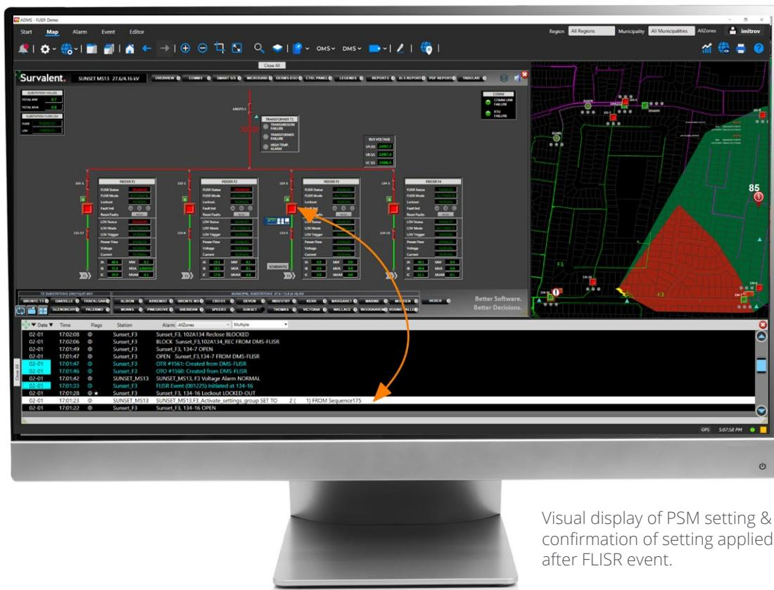
Visual display of PSM setting & confirmation of setting applied after FLISR event.
