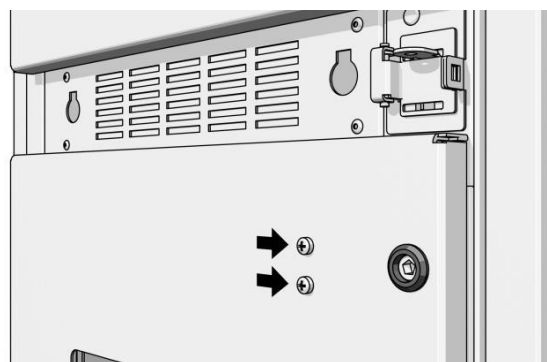
Fig. 4-14 Interlock defeat mechanism screws
