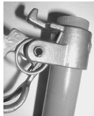
FUSEHOLDER IS AVAIL- ABLE WITH A TORSIONAL SPRING ON TRUNNION TO AID DROP OUT OPERATION IN CORROSIVE ENVIRON- MENTS.
