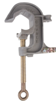
C6002256 Aluminum body, Serrated jaws, Bronze eyescrew with Acme threads, Tapped for 5/8-11 UNC threaded ferrule or PSC6003412, Drilled for 5/8-11 UNC threaded ferrule *Unshrouded Ferrules Only
