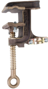
C6002232 Bronze body, Serrated jaws, Bronze eyescrew with Acme threads, Drilled for 5/8"-11 UNC threaded ferrule or T6003196, Tapped for 5/8"-11 UNC threaded ferrule or PST6003485 for Fine Thread Eyescrew version
