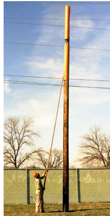
When space is extremely limited for truck storage, a 23 ft. Telescoping Tool that compacts to 4 ft. is available as Catalog No. C4031739.
