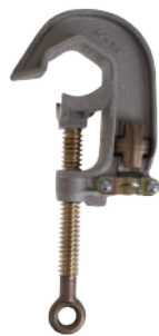
C6002282 Aluminum body, Serrated jaws, Bronze eyescrew with Acme threads Bronze pressure-type terminal
